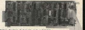
F) FLOPPY DISK DRIVE ADAPTER *Connects main board with floppy disk drive. *One card can handle four floppy disk drives without any adjustment. *With Printer Port
